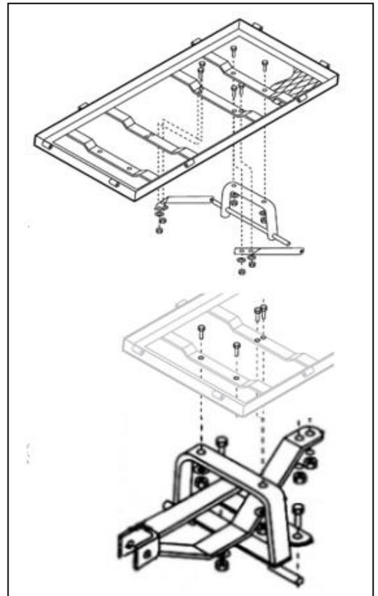
**C.** Attach the Steering Yoke (11) to the centre of the Front Axle Assembly using the washer and split-pin and washer already attached to the mounting post. Next secure the axle Support and steering link connector using (19) 8x20mm bolts, (17) 8mm lock nuts, and (16) 8mm washers (as shown in Figure 2)
